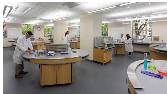
University of Illinois Urbana-Champaign Chemistry Building Labs implement oval air stations to keep line of sight clear in the instructional lab.
